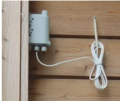
Figure 19: Adeunis Temperature sensor installed on USN campus.
